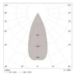
Correlated color temperature: 3000 – 6000 kelvin Rated median useful life: 50000h L70 at 25°C Luminaire input power: 3 w
